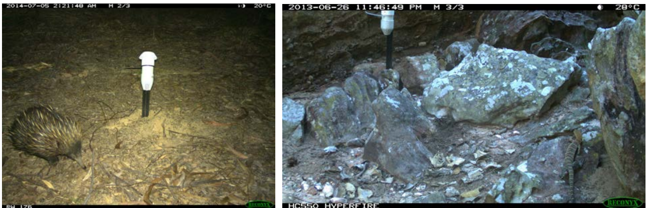
Figure 21: Examples of a correct and incorrect positioned camera and bait station. In the left image the site is well cleared of vegetation and the base of the bait station is in the centre of the frame, ensuring that any small animals approaching the bait station will be photographed. In the right image the bait station is not centred, resulting in the base of the station being located outside the sensor zone. The large rocks in the field of view will potentially impede detection of animals. However, note the Kimberley Rock Monitor ( Varanus cf. glauerti ) in the bottom-right corner of the right image.
