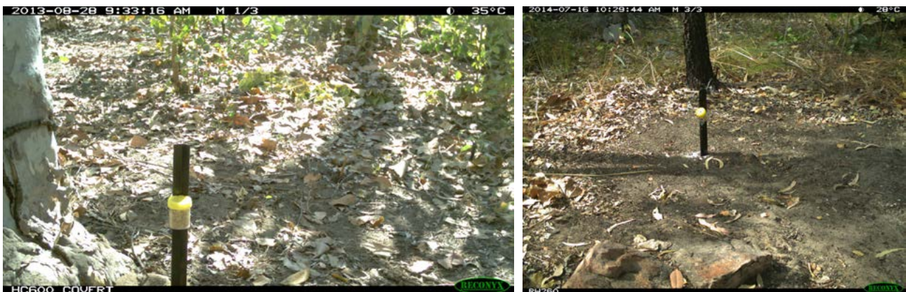
Figure 14: The image on the left shows a poorly prepared camera station; vegetation has not been cleared, the bait station is not centred and the base of the station is not in frame. The image on the right shows a well prepared set up.
