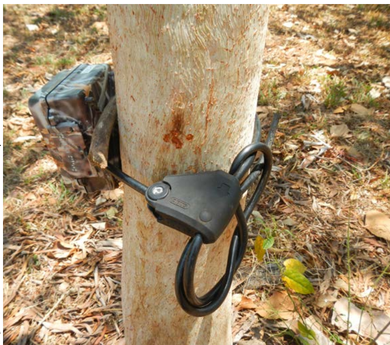
Figure 9: Camera secured to a tree with a bike cable lock.
