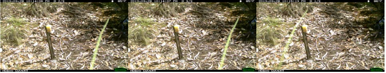
Figure 12: False triggers caused by a single blade of grass moving in the sensor view.
