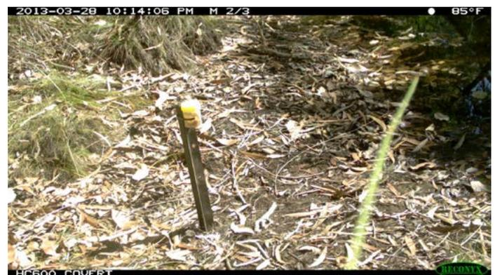
A false trigger caused by a single blade of grass moving in the sensor view.
