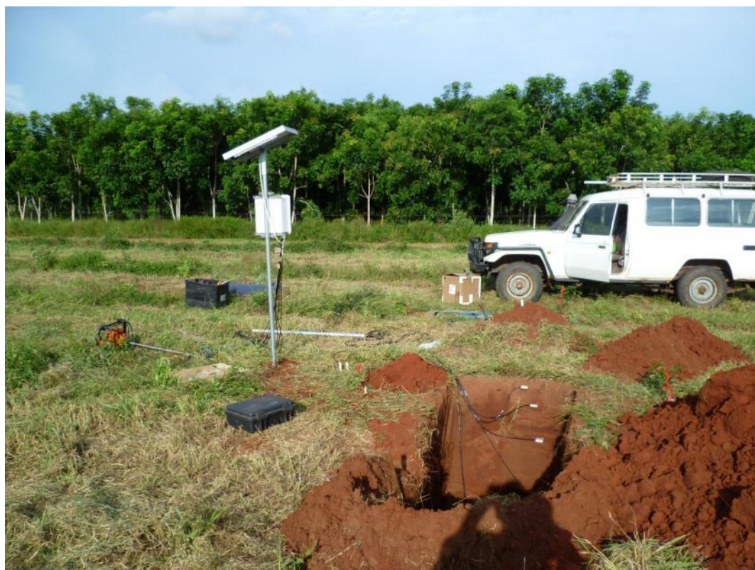
Figure 11 High density planting bay at the DDRF as of March 2011 during soil moisture pit installations. Probes were inserted in the pit wall which was then backfilled. Each soil pile was
