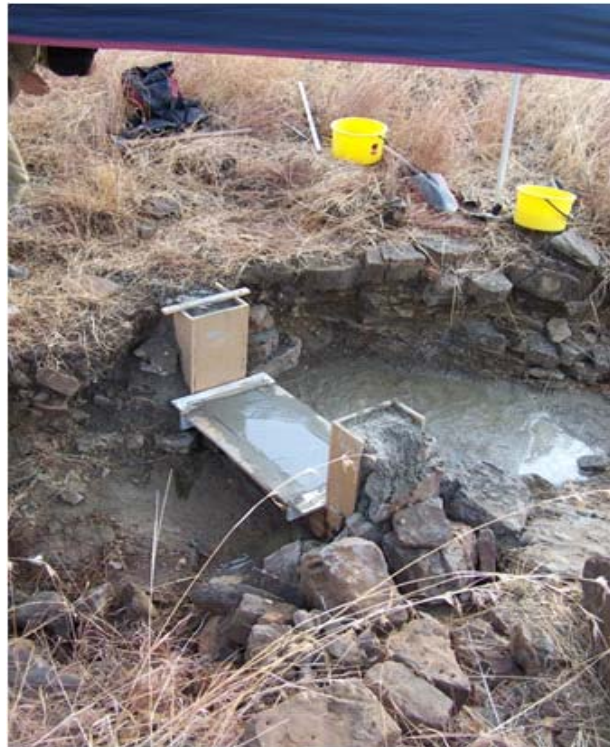
Plate 6-3 Mini-flume construction, November 2009 at the PCA site, Florina Rd, Florina, NT. The catchment was approximately 2.6 ha, consisting of undulating hills with shallow, rocky, skeletal soils. Photo, M. Northwood.
