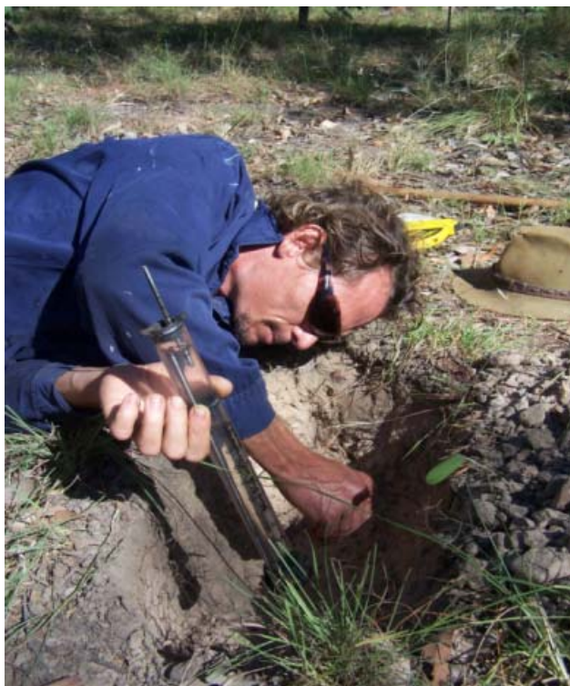
Plate 6-2 Careful preparation of the soil horizon at 30 cm for mini-disc infiltrometer measurements
