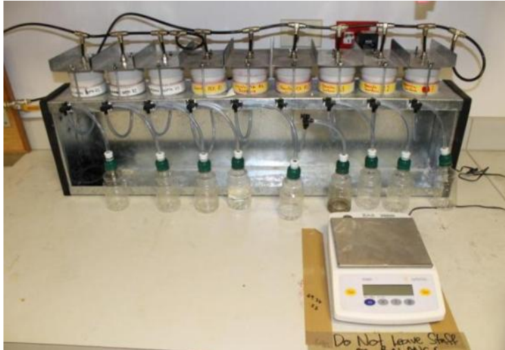
Plate 6-1 Tempe cells designed and constructed at CDU's ecophysiology laboratory to determine the soil moisture characteristics for each soil type over a 0.1 to 1 bar pressure range. Using this apparatus, nine samples can be tested simultaneously at two pressures.
