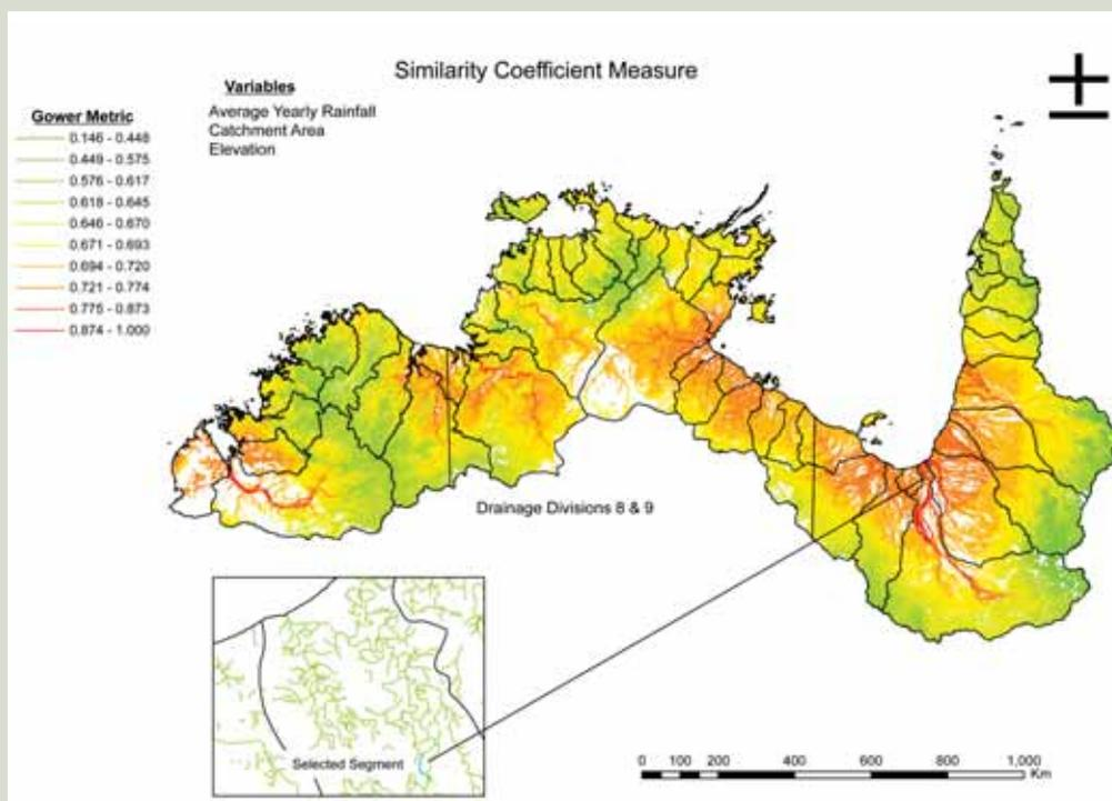
**Figure 1.** The GIS-based geomorphic classification tool highlights that there are major differences between rivers in the Southern Gulf country and in the Kimberley. In this example, streams that are similar to the selected section of river are shown in red. Streams that are dissimilar are shown in green.
