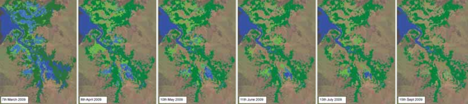
Figure 2. Flood inundation for the Daly catchment floodplain in 2009, captured using satellite imagery. Surface water and seasonal grasses contract from the end of the wet season (March) to the end of the dry season (September).
