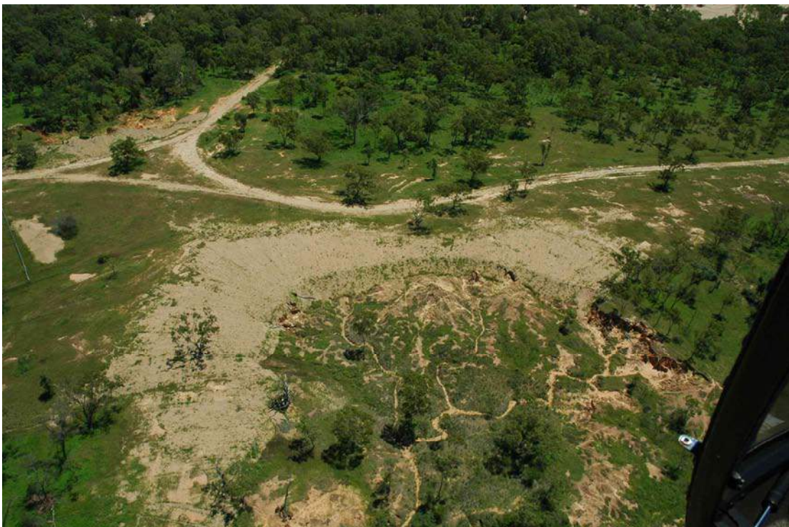
Figure 7-7 Oblique aerial view of a gully head scarp at Mount Mulgrave that has been backfilled with local river sand in an attempt to slow erosion into the road in the background. Note the original scarp front remains intact in the right side of the photo.
