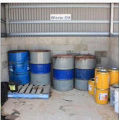
Waste oils stored in bunded shed Pormpuraaw Aboriginal Shire Council, Sept. 2016
