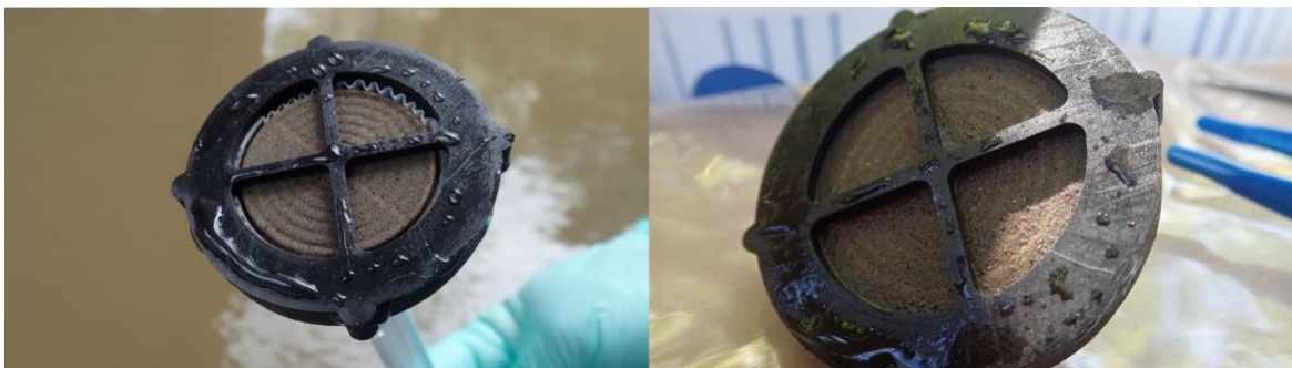
Figure 6. 20 \mu\text{m} nylon net filters in 3-D-printed cartridges clogged with suspended sediment.
