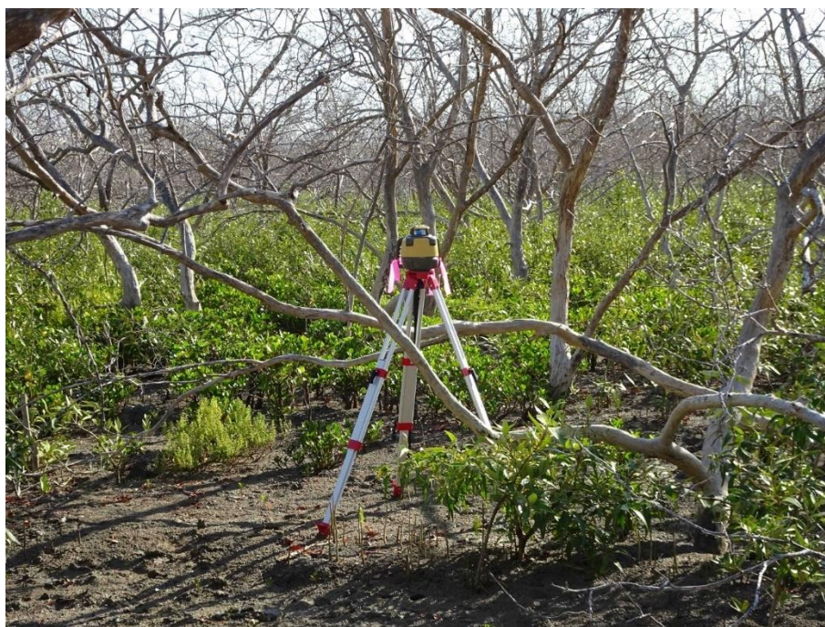
Figure 2.6. Elevation levels were made using a Topcon rotary laser with a range of around 500 metres depending on the density of vegetation.
