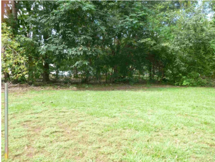
Figure 7. Correct alignment of a sighting dropper for a site photo – its base in the bottom left hand corner of the field of view.
