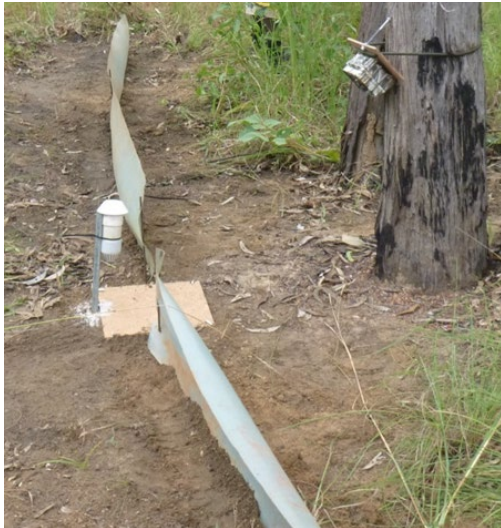
Figure 6. Bungee strap and mounting screw used to angle camera to focal point at centre of the corkboard.
