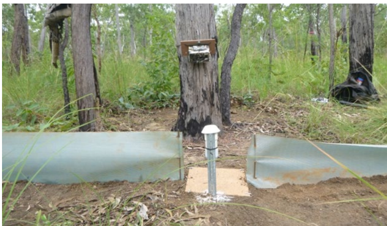
Figure 7. Correct drift fence, bait station and camera deployment arrangement for RS cameras.
