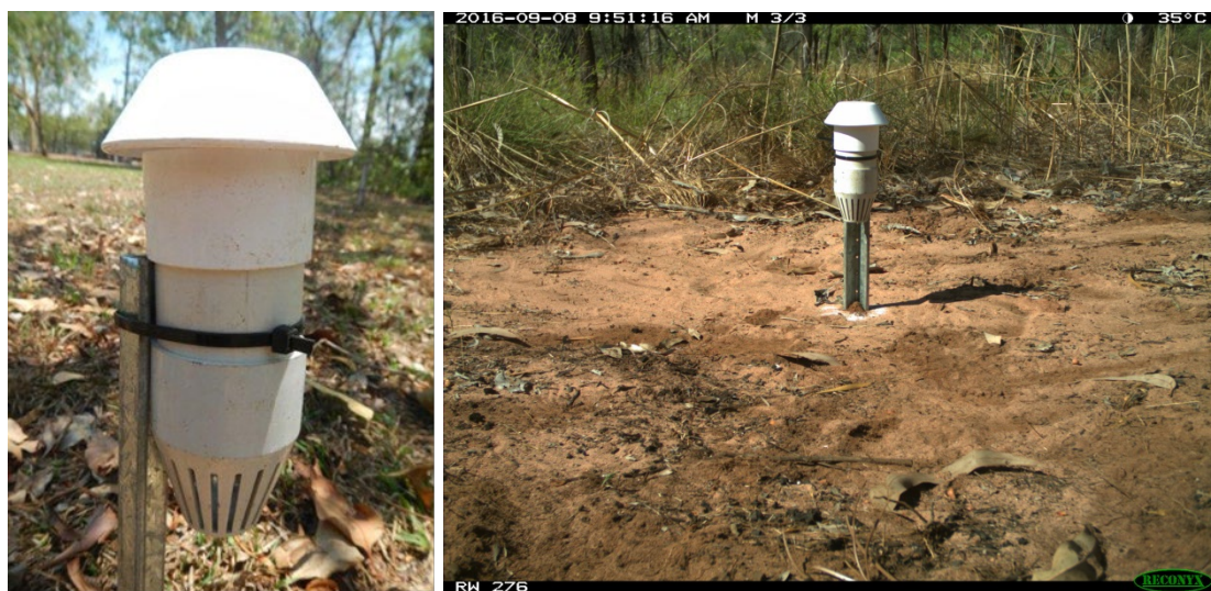
Figure 9. Bait station secured to stake with a cable tie (left). Ant granules are visible around the base of the bait station (right).
