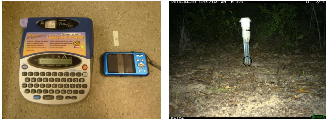
Figure 2. Digital camera with label placed on viewing screen (L) and camera trap image showing (R) the positioning of the base of the bait station within the optimal (black circle) location. This may vary for camera models so test each camera with a reference model in order to attach the transparent label correctly.
