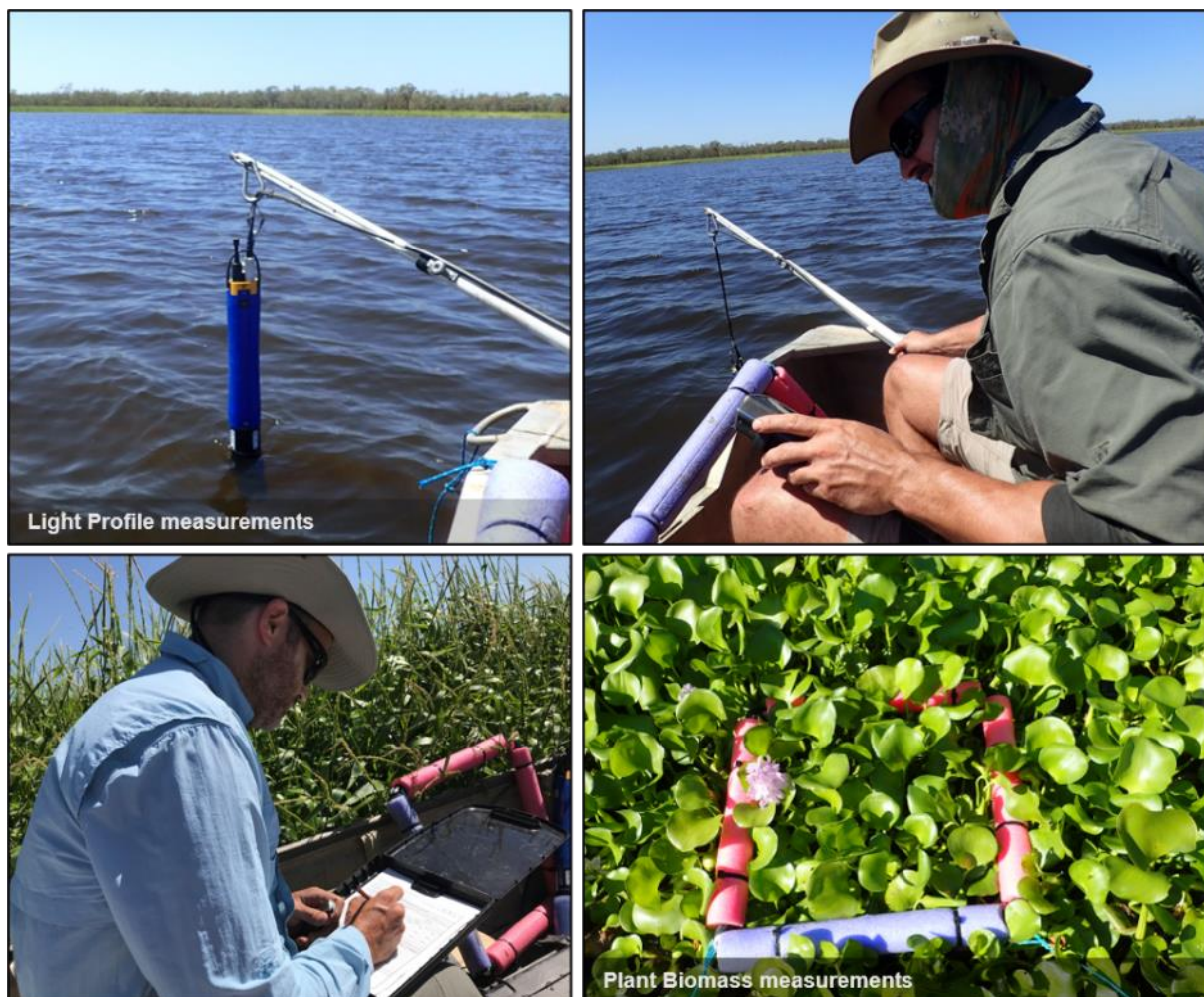
Figure 3-3. Collection of photosynthetically active radiation profile and plant biomass. Photos: Bianca Molinari.
