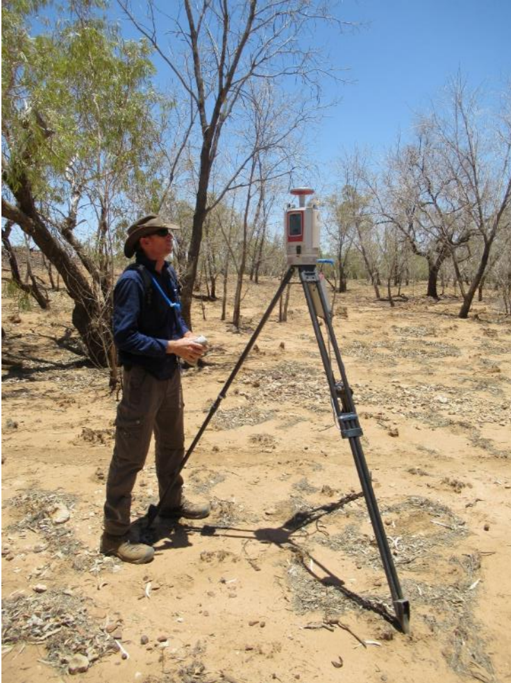
Figure 4. The Riegl VZ-2000i terrestrial laser scanner in use.
