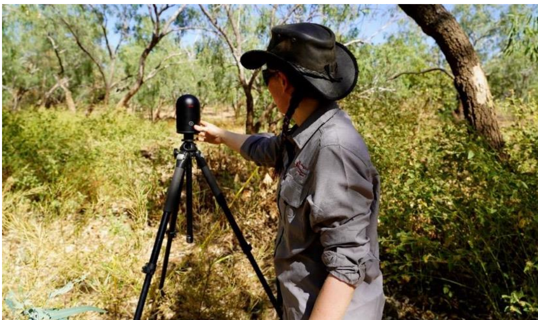
Figure 9. The Leica BLK360 in use. Photo: Karen Dayman.
