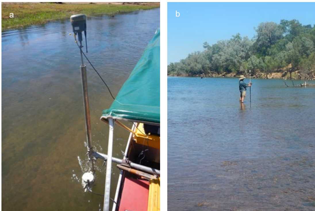
Figure 3-3. (a) Bathymetric survey equipment, and (b) survey of non-navigable areas.
