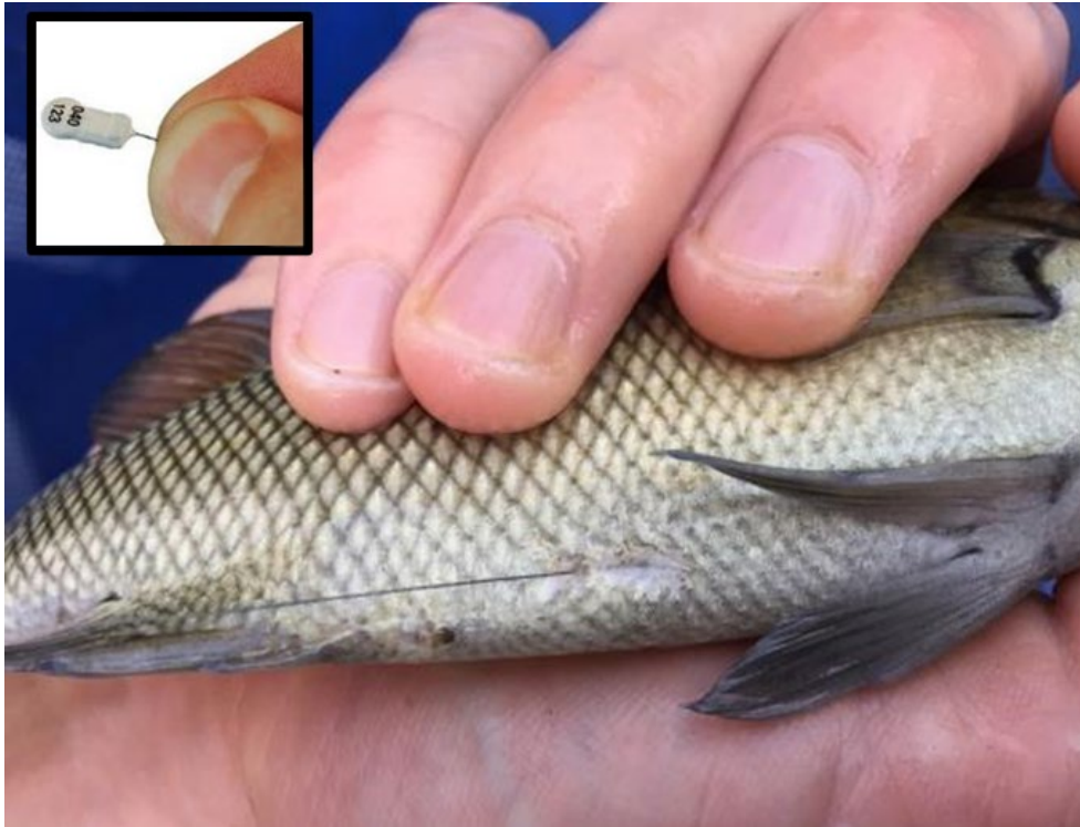
Figure 6-4. Radio-tagged juvenile sooty grunter showing trailing antenna; inset shows size of transmitter.
