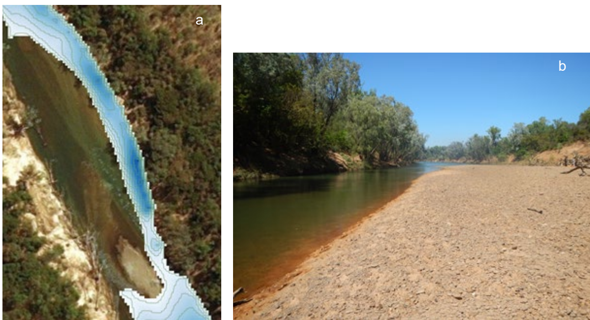
Figure 3-6. (a) Modelled upper riffle in Mentabie Reach showing the modelled outputs overlaying a pre-September 2014 satellite image of the area; (b) The large sandbank that had established at the same location by 2017 when the bathymetric work was undertaken.
