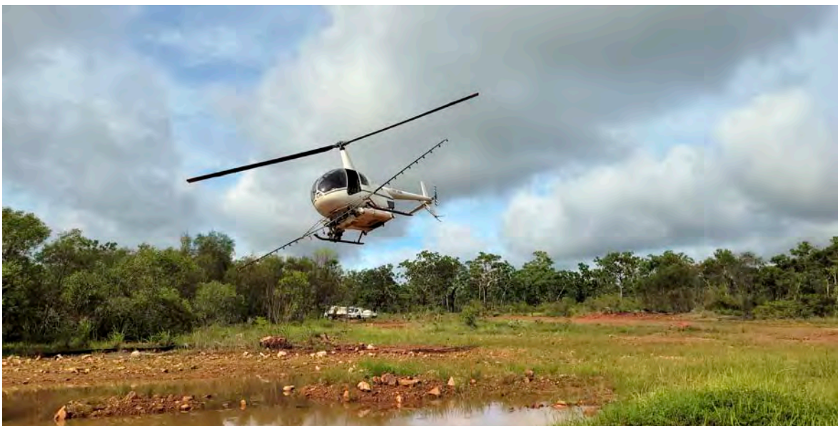
Helicopter equipped with a boom spray unit in Lichfield National Park for spraying large, dense gamba grass infestations.
