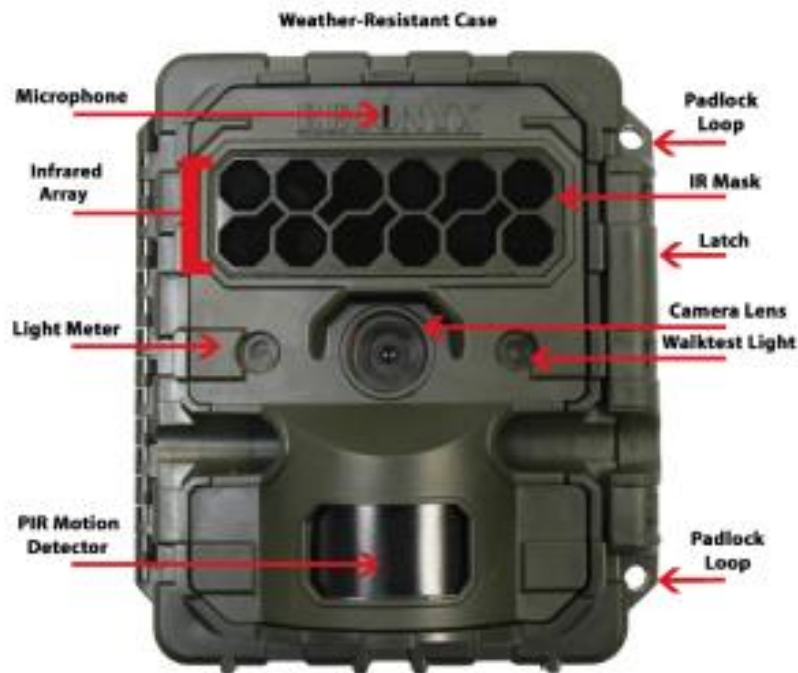
Figure 3. The components of a Reconyx HP2X. The Fresnel lens and PIR are described here as a PIR Motion Detector. Image courtesy of Reconyx.
